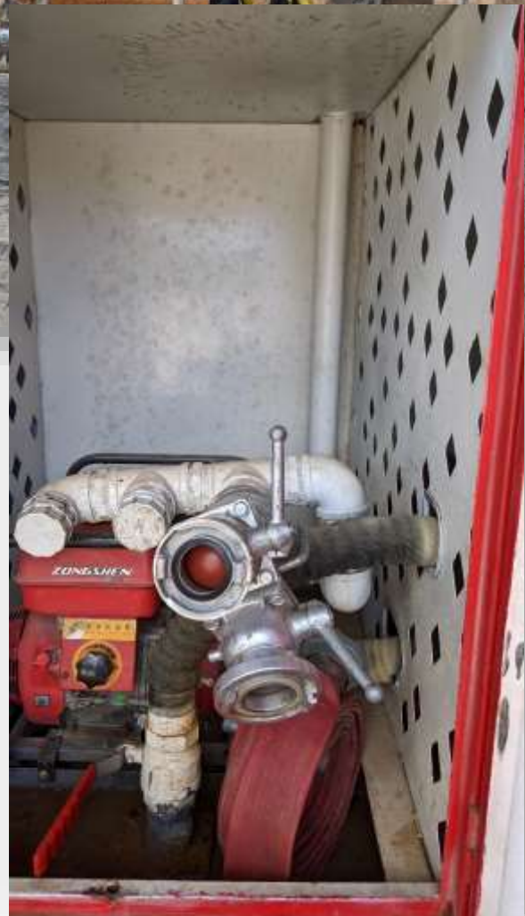
13 special construction; divider with adaptor für connectin german and chinese couplings
